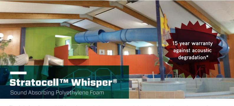
**The Solution:** Stratocell Whisper®, a revolutionary new sound absorbing material was chosen to fix the problem. Stratocell Whisper is ideal for indoor and outdoor environments where reverberant noise is a problem. 100 lightweight panels were fitted at strategic positions in the pool area.
